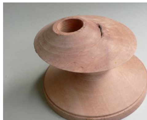
Inside – outside Turning and then offset turned.
