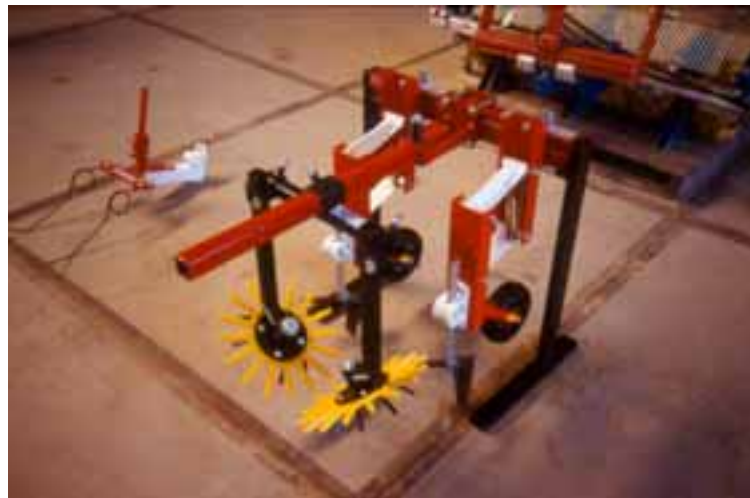
Figure 2: Set of new finger weeders on the right with a pair of torsion weeders on the left.
