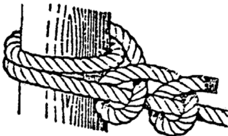
Figure 6-5 Round turn and 2 1/2 hitches
