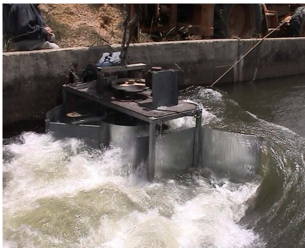
Testing the Sundermann turbine in an irrigation channel
