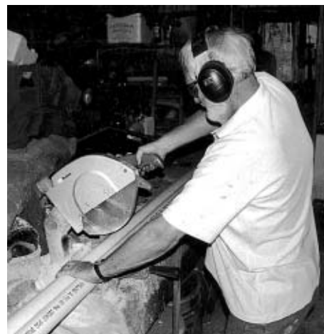
Friends of Hattah-Kulkynne cutting the plastic tubing into 800 mm lengths – a step in their production of 1000 Carroll tubes to be used in their tree-planting project.
