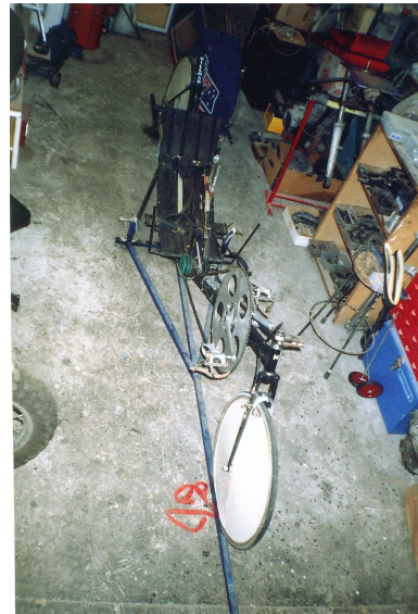
Recumbent frame on new support frame, December 2005. Note new 24" tubular front tyre.
