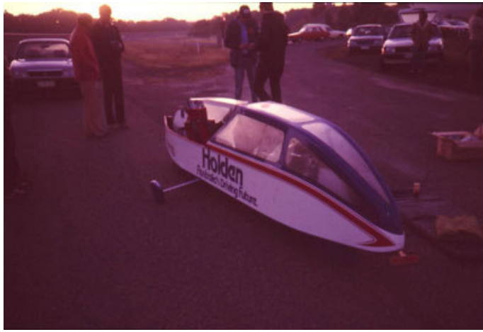
Lang Lang test track, dawn, 28 March 1984: GMH technician makes final checks of HPV cockpit instrumentation. Note near-side outrigger wheel.
