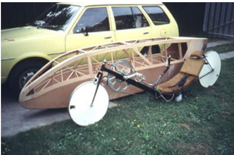
Lachlan Thompson HPV under construction at Bayswater, early December 1983. Vehicle frame is fully assembled except for high-pressure tyres and outriggers. Note caliper brakes on rims, toe-clips, and joystick control.
