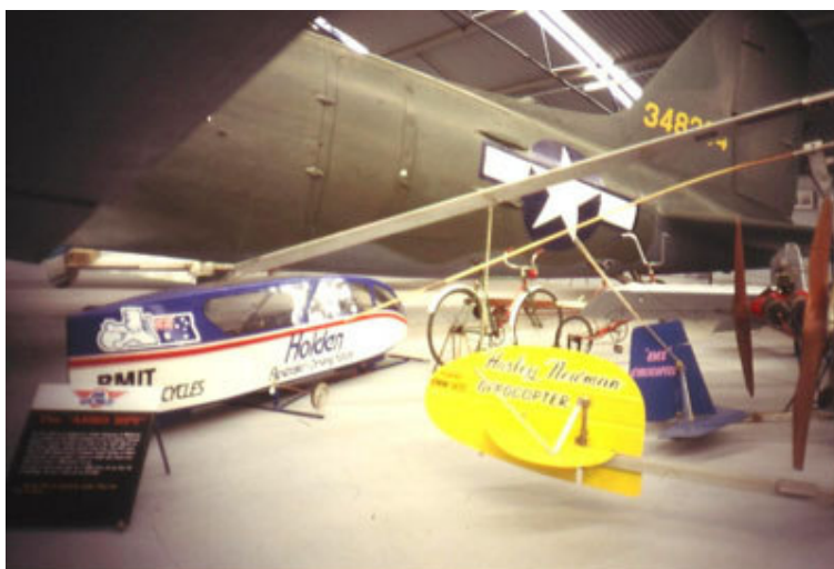
The HPV at Drage Airworld, March 1997. Note steel support frame and non-authentic outrigger wheels.
