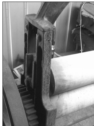
Original red edging was exposed on the cast iron frame and gear
